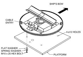
Figure 5-4 Antenna Unit, cover removed
